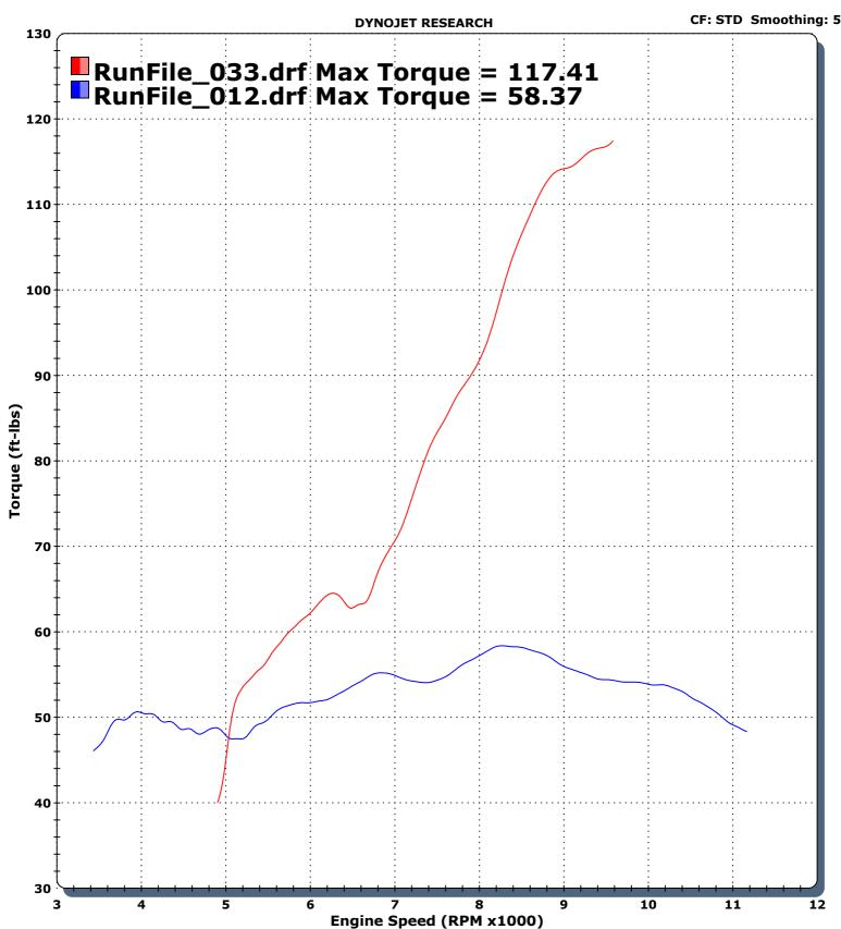
RunFile\_012.drf - 09/08/2010 17:07:27 Run Type: RO Run Conditions: 21.14 °C, 30.48 in-Hg, Humidity: 42%, STD: 0.99 Max Torque = 58.37 Ducati 749 2005.Racebike, Termi full system, Race intakes, Hi-flow filters, lightend flywheel.. Powercommander and both cyls Dyno-Tuned Tuned by Bunbury Dyno. 7k on +5%
