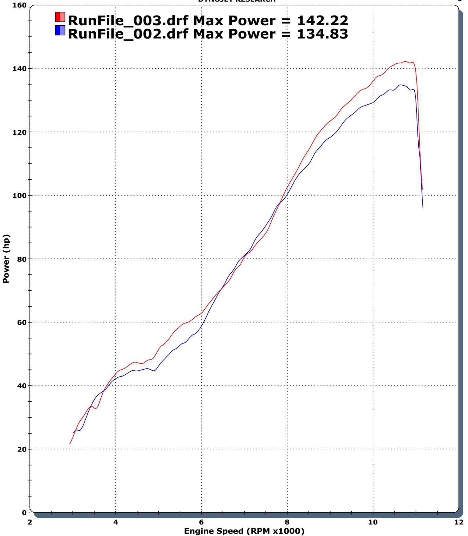
RunFile\_002.drf - 04/02/2011 14:48:53 Run Type: RO Run Conditions: 35.64 °C, 29.87 in-Hg, Humidity: 29%, STD: 1.04
