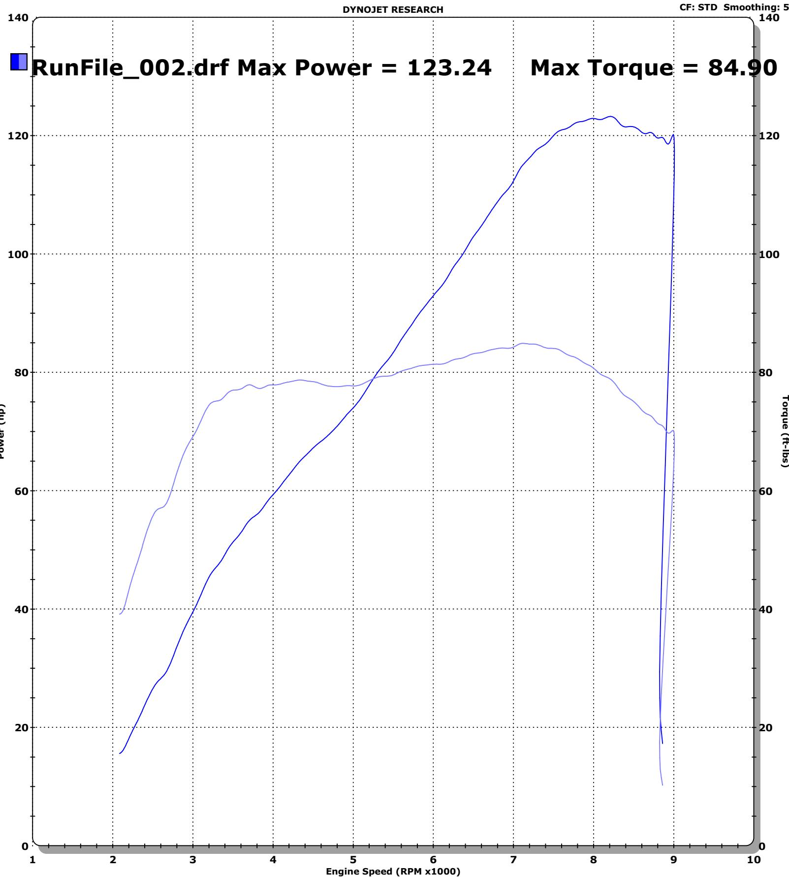
RunFile\_002.drf - 8/04/2009 11:54:40 AM Run Type: RO Run Conditions: 83.44 °F, 30.23 in-Hg, Humidity: 25%, STD: 1.01
